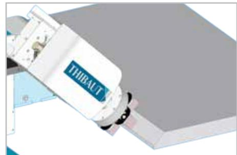
**Polishing of thick inclined straight edge.**
