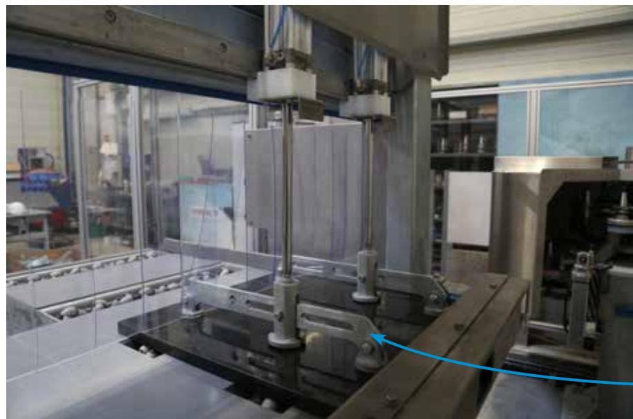
+ The assembly and disassembly of the clamping beams is carried out without tools.
