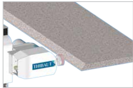
Polishing of thin straight edge.
