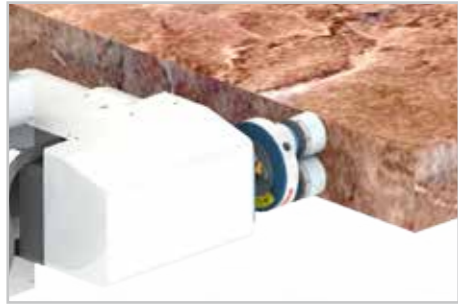
Thick straight edge polishing.
