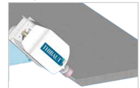
Horizontal arrise polishing.
